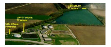
Photo 4-1 Aerial Photo of LaPorte wastewater treatment facilities showing flow meters
