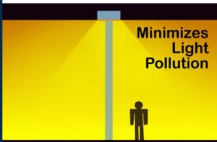
Utilize cut-off fixtures to minimize light pollution and off-site glare
